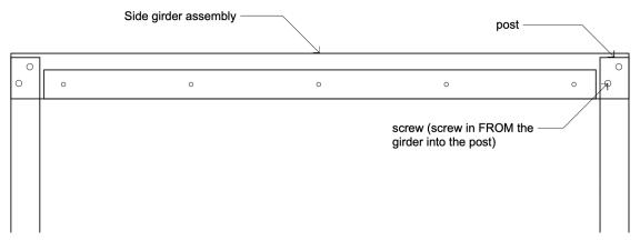
For this part, you will need a friend. Posts should align to ½" from the top of the 2x6 girder and are flush to the edge. Start on the ground - measure & attach the side girder assembly (start with only ONE screw connecting the post to the side girder) to two posts and raise it to form a frame. Use your level to ensure that when you raise the frame, the posts maintain plumb and the girder is level. Once you are happy, screw in your second screw.
