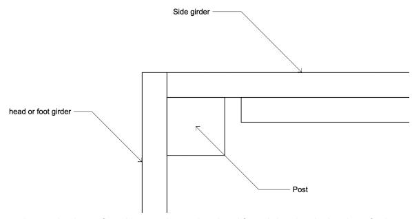
Once you have raised your first side, attach your head and foot girders by placing them flush with the side girder. They should stick out to 'complete' the corner, as seen in the birds-eye picture above. When attaching them, make sure to use the level to maintain proper alignment.
