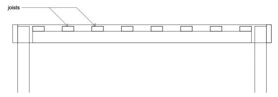
This should be the easiest part! Joists are cut  $\frac{1}{2}$ " short of the length of the gap and should rest on the joist rail with ease. Space them evenly to support your mattress. You can optionally screw them down into place, but this is not necessary.
