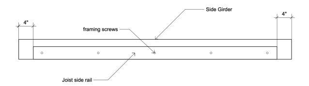
The joist side rail should be attached exactly (horizontally) centered and flush with one long edge of the side girder. This means there should be a 4" distance on both sides between the side rail and the girder. Screw in 5 framing screws connecting these two pieces. Repeat again for the second side rail.
